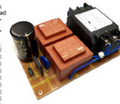
Figure 16 UPS protection system and its voltage detector
