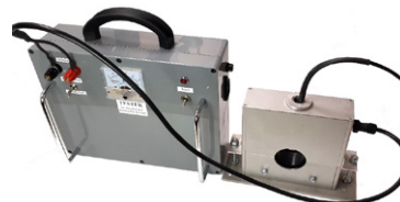
Figure 11 Simple E3 component simulator for testing serviceability of the system for protection of high-power transformer
