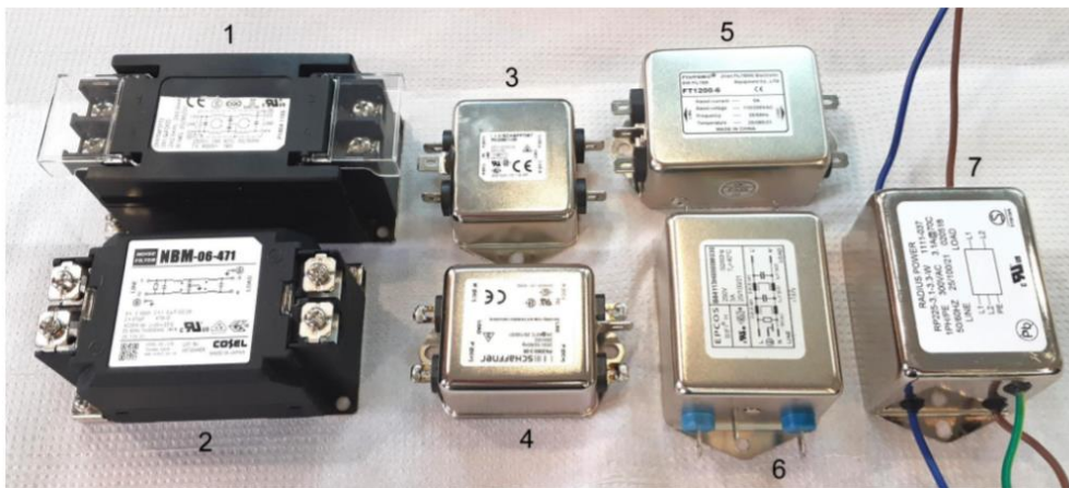
Figure 6: Two-stage EMC LC-filters of various types with improved specifications: (1) 62-MTB-060-4-21 (API Technologies); (2) NBM-06-471 (Cosel); (3) FN2090-1-06 (Schafner); (4) FN2060-3-06 (Schafner); (5) FT1200-6 (Jinan Filtemc Electronic Equipment); (6) B84113H0000M030 (Epcos); (7) RP225-3.1.3.3-W (Radius Power).
