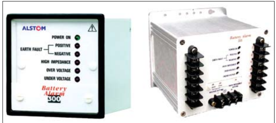
Fig. 1: Device BA300 type (Areva) for constant monitoring substation battery impedance, voltage and ground insulation levels.
