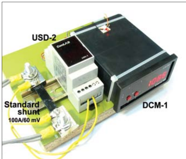
Fig. 5: Model of the system based on standard shunt for supervision battery circuit. USD-2 – electronic transducer (input: \pm 200 \mu V , output: 4 - 20 mA); DCM-1 – programmed electronic transducer for 4 - 20 mA with relay output (Conlab, Israel).
