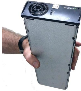
Fig. 3. Compact BCs with intermediate high frequency link. Variable output voltage: 60V or 67V, output current up to 30A.
