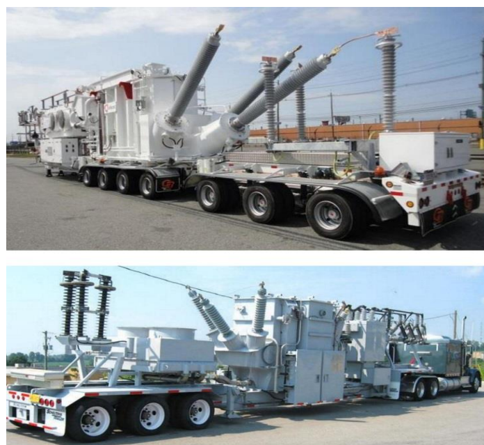
Fig. 1. Several types of mobile substations
