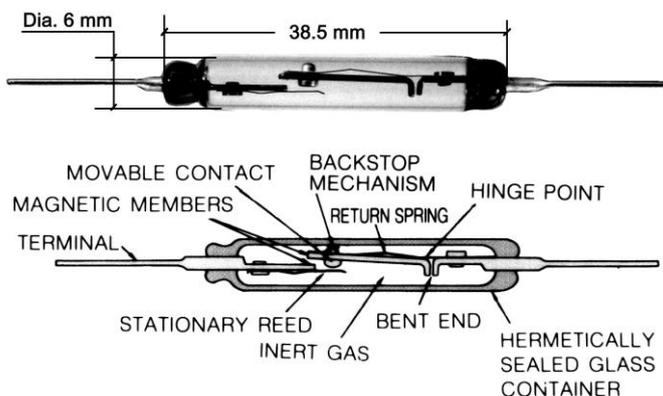
Fig. 4 A powerful gas-filled reed switch Bestact R15U by Yaskawa Company with a two-stage switching
