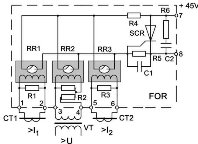
Fig. 2 Starting unit (SU) based on hybrid Fast Overcurrent Relay
