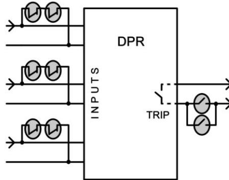
Fig. 1 Application of EMPR based on high speed reed-switches to shunting sensitive inputs of DPR and block its output (trip) contact
