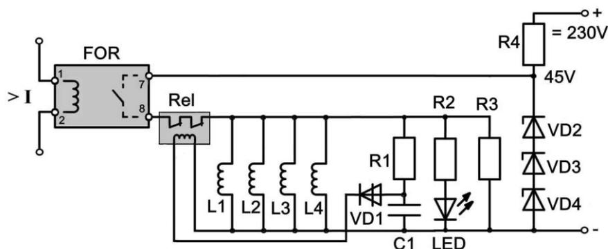
Fig. 3 A diagram of connection of final control reed relays (L1 – L4 – control windings of these relays the contacts of which are shown in Fig. 1)
