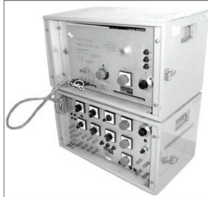
Fig. 2: Advanced test set TURH-20 type (ASEA) for testing of electronmechanical protective relays containing sets of inductances and resistances
