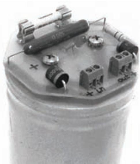
Fig. 4. The prototype of the device for reserve feed of MPR.
