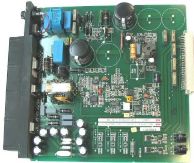
Fig. 2 - The PCB of the switching power supply of the MBR, combining SMD microcomponents with large discrete elements of usual installation.
