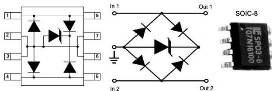
Fig. 6. Transient voltage suppressor diode (TVS) SP03-6 type.
