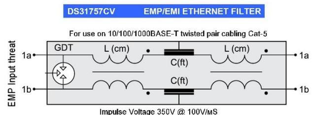
Fig. 2. Circuit diagram of a device protecting Ethernet network from HEMP based on gas discharge tube (GDT) manufactured by MPE Company.
