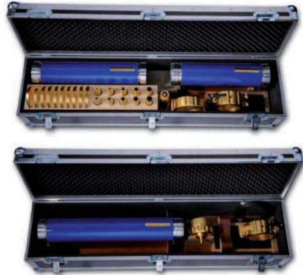
Fig. 8: A kit of testing tubes (type CoMeT 90/1) with a kit of locks and connectors manufactured by the Bedea (Rosenberger) company to test cable shielding effectiveness with an outside diameter from 6 through 22 millimeters.
