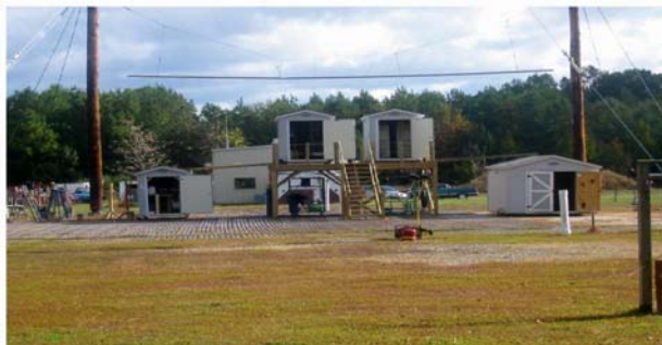
Fig. 6. Testing of SCADA system for immunity to HEMP [7]. An antenna system of EMI simulator is seen above. The elements of SCADA system are located in separate boxes and connected with each other via a standard communication system
