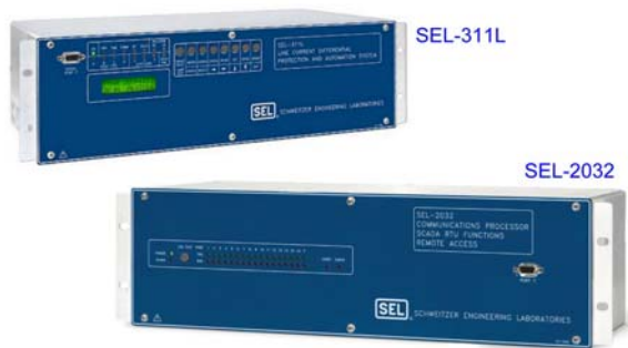
Fig. 1. SEL-311L DPR and SEL-2032 controller for SCADA system produced by Schweitzer Engineering Laboratories (USA) subject to testing for HEMP immunity
