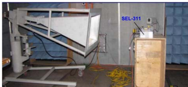
Fig. 2. SEL-311 DPR test for IDEI impact on Picatinny Arsenal test-benches in New Jersey [6]
