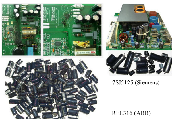
Fig. 2. Faulty DPR switched-mode power supplies of different types with damaged electrolytic capacitors, left figure shows taints in printed circuit boards from electrolyte leakag.
