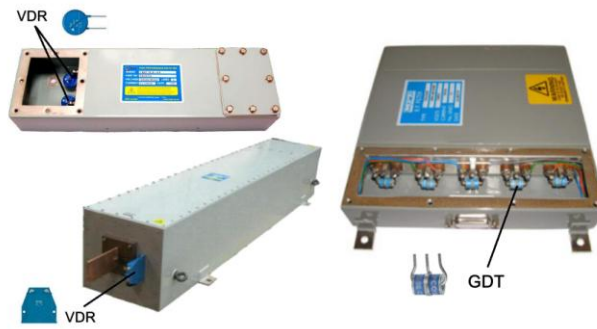
Fig10. HEMP filters manufactured by the MPE company, which include voltage depended resistors - VDR (varistors) and gas-discharge tubes (GDT) as elements protecting from high voltage pulse
