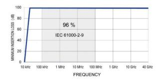
Fig. 11. Typical amplitude and frequency features of HEMP filters represented in ETS-Lindgren's promotional materials.
