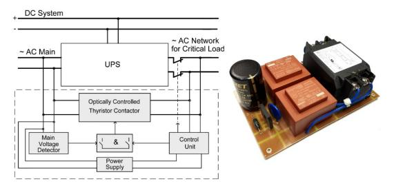
Fig. 33. UPS protection system and it's voltage detector
