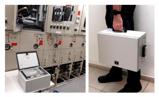
Fig. 31. HEMP protected backup power supply for electronic equipment testing after HEMP impact
