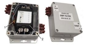
Fig. 25. HEMP power line filter for microprocessor-based protection relays inside the control cabinet. 1 – special high-efficiency surge arrester; 2 – electromagnetic two stage filter.
