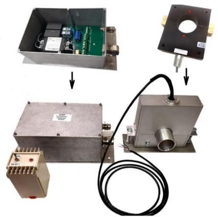
Fig. 27. Simple system for protection of high-power transformer against E3 component of HEMP
