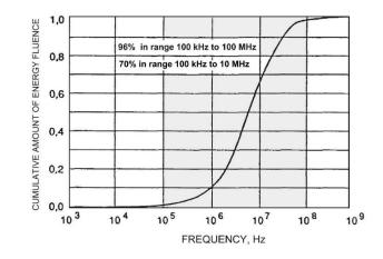
Fig. 13. HEMP energy distribution over the frequency range (see IEC 61000-2-9 [10])
