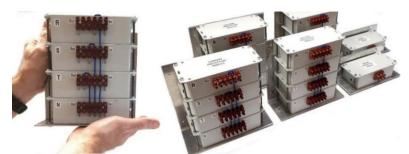
Fig. 24. Special HEMP filters designed by author for installation in current and voltage circuits of microprocessor-based protection relays
