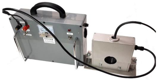
Fig. 28. Simple E3 component simulator for testing serviceability of the system for protection of high-power transformer
