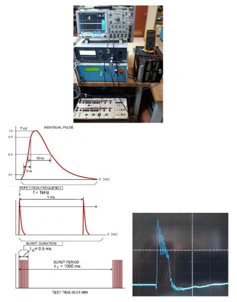
Fig. 6. Testing equipment and set-up of the Electrical Fast Transient (EFT) pulse generator (EFT is very close in shape and duration to HEMP) to test compliance with IEC 61000-4-25 and oscillogram of the real pulse.
