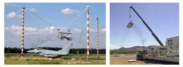
Fig. 19. Hybrid-type HEMP simulators: stationary (left) and mobile (right).
