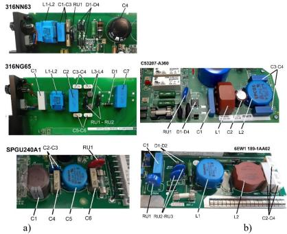
Fig. 7. Various types of input filters on DPR's power supplies, a) manufactured by ABB; b) manufactured by Siemens. In addition to capacitors C<sub>N</sub> and chokes L<sub>N</sub> of the filters, also include varistors RU<sub>N</sub>.
