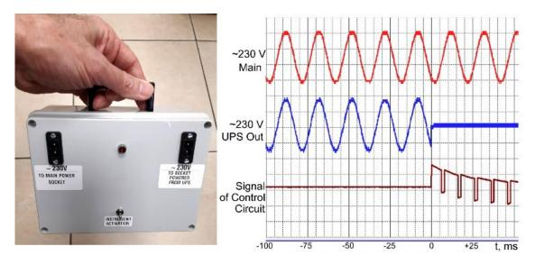
Fig. 34. Simple tester for express verification of the serviceability of the UPS unit after the HEMP impact.
