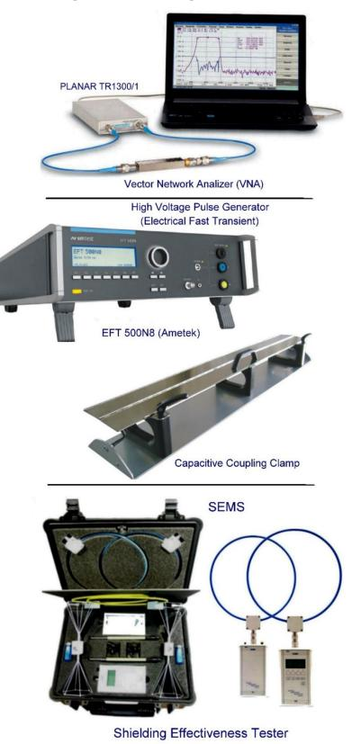
Fig. 20. Instruments sufficient to test civilian equipment for resistance to HEMP.
