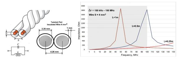
Fig. 5. Estimation model for a twisted pair of conductors and impedance of a twisted pair of mounting wires of different lengths (1 m; 0.5 m; 0.25 m) as a function of frequency.
