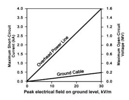
Fig. 23. Voltage and current induced in long overhead lines and ground cables by E1component of HEMP from kiloton-class yield weapons.
