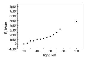
Fig. 21. Changes of the electric field intensity at different HOBs over the explosion center for 1Mt yield [15].
