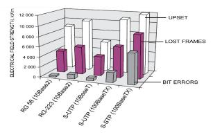
Fig. 9. The level of susceptibility (failures) of the simplest computer network for various network and cables configurations.
