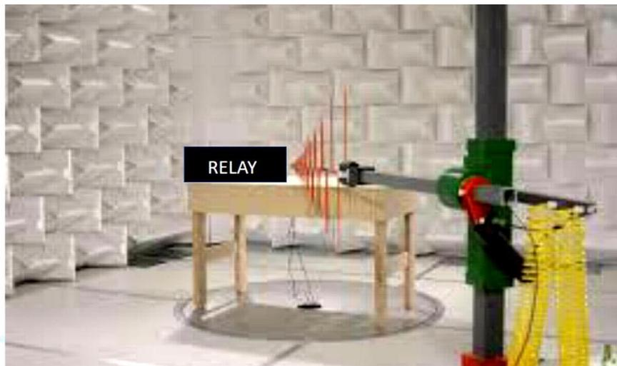
IEDs have Passed the Radiated 50kV/m EMP Test
