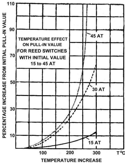
Fig. 4. Impact temperature on pickup current (pull-in value) for reed switches with various initial sensitivity (ampere-turns or AT)
