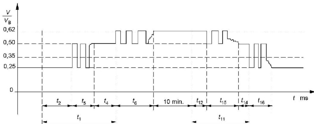
Fig. 6. Oscillograms of switch-on and switch-off processes in the reed switch
