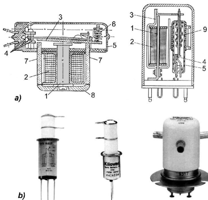
Fig. 1. Design of electromagnetic (*not reed switch*) relays with hermetically sealed contacts placed in gas filled or vacuumized shell (a) and external view not reed switch relays with hermetically sealed contacts (b) manufactures by companies Kilovac, Jennings, Gigavac.
