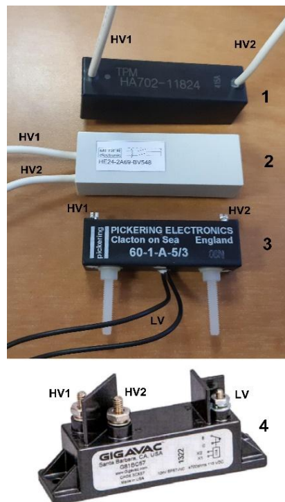
Figure9. High-voltage reed switch relays selected for impulse insulation strength test. 1 – type HA702-11824; 2 – type HE24-2A69-BV548; 3 – type 60-1-A-5/3; 4 – type G81AB47. HV1 and HV2 – outputs of high-voltage reed switch, LV – outputs of low-voltage control coil.
