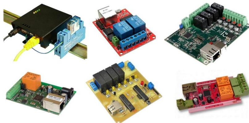
Figure7. Network relays with a different number of channels and output electromagnetic relays.
