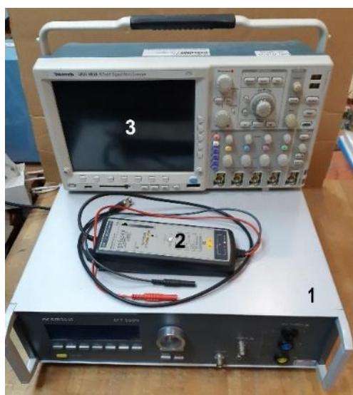
Figure2. Equipment used during the test. 1 – Generator of short high-voltage pulses (Electrical Fast Transient) EFT 500N (Emtest) with output voltage up to 7 kV, 2 – active differential high-frequency high-voltage probe TA044 (Pico Technology), 3 – oscilloscope MSO 4034 (Tektronix).
