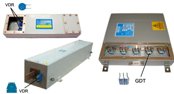
Fig. 3. Filters of the MPE Company with protective elements consisting of voltage dependent resistors – VDR (zinc-oxide varistors) and gas-discharge tubes (GDT) at inputs
