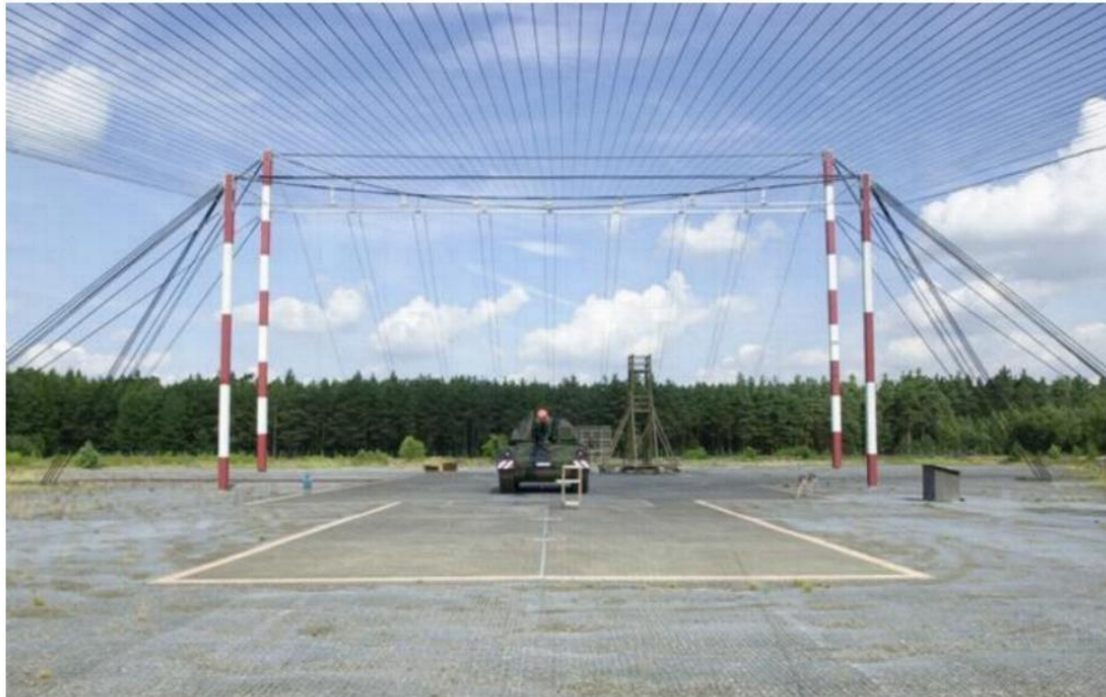
Fig1. Design and appearance of HEMP simulator.
