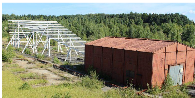
Fig4. Stationary HEMP simulator ALLUR of High-Voltage Scientific-Research Center of Federal State Unitary Enterprise Russian National Electric Technical Institute (Istra, Moscow Region). Overall dimensions: 100m x 35m x 13.5m; displacement volume: 10m x 10m x 10m; pulse shape: 2.5/25 nanoseconds; maximum strength of electric field pulse: 70 kV/m.
