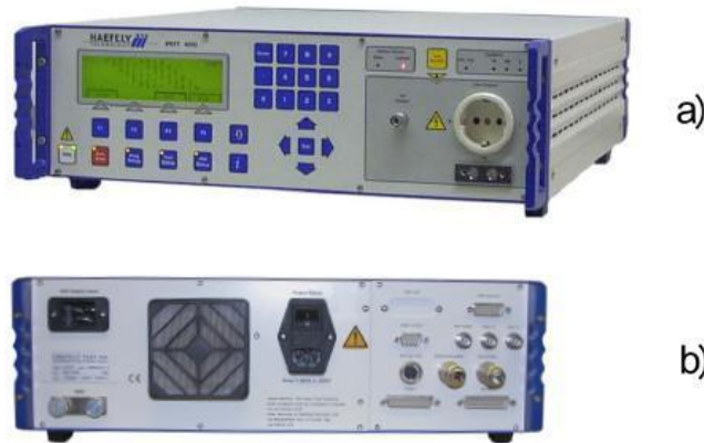
Fig6. EFT generator type PEFT 8010 with the maximum pulse amplitude of 7.3kV, manufactured by Haefely EMC Technology (Sweden), a – front panel view, b – rear panel view.
