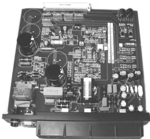
Fig. 4. Built-in switching power supply.
