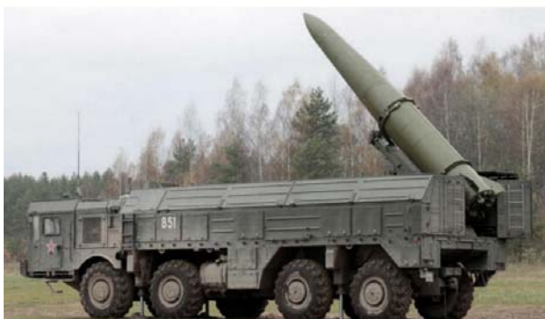
Fig. 3. Missile launchers of a battle-field support rocket SS-21 «Scarab B» (Tochka-U) – above and tactical ballistic missile system SS-26 «Stone» (Iskander-E) – below
