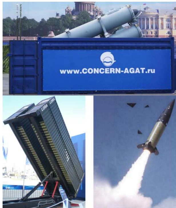
Fig. 4. Container-based launching units of missile complexes Club-K (above) and LORA (below)
