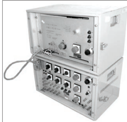
Fig. 2: Advanced test set TURH-20 type (ASEA) for testing of electromechanical protective relays containing sets of inductances and resistances
