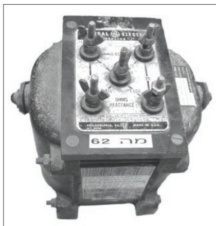
Fig. 1: Set of inductances from General Electric for testing of electromechanical protective relays
