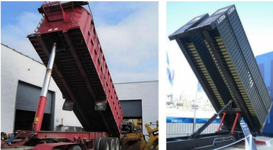
4. A conventional shipping container (left) and a LORA missile system container (right). Source: Vladimir Gurevich, PhD
