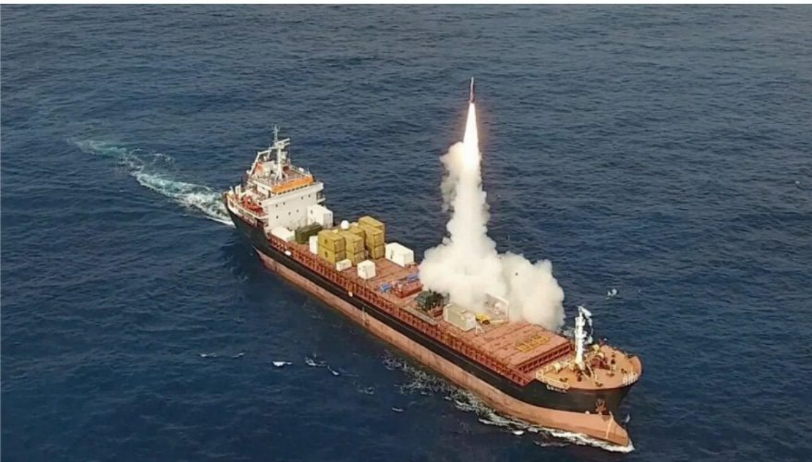
5. An ordinary civilian container ship loaded with hundreds of standard containers (top), and a LORA rocket launched from a container ship during a test (bottom). Source: Vladimir Gurevich, PhD
