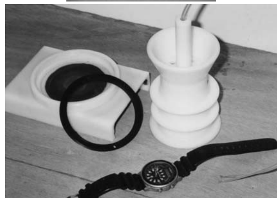
Fig. 11. External view of high-voltage (24 kV) overcurrent reed relay not requiring CT
