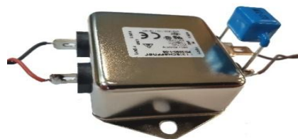
Figure8. Two-Stage Electromagnetic Filter FN 2090-3-06 Equipped With a Powerful TVS-Diode MAX-370 Type on the Input
