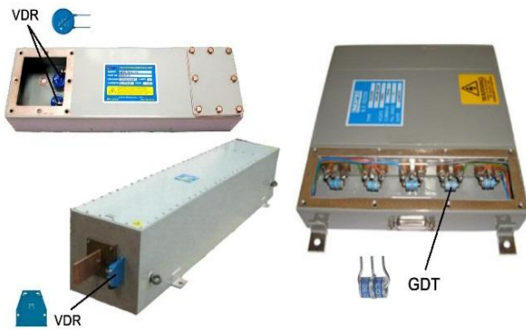
Fig.6. Some HEMP filters equipped with HV pulse protecting elements. VDR – varistor, GDT – gas-discharge tube.
